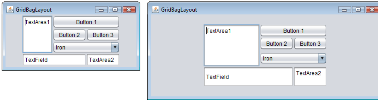
Fig. 22.20 | GridBagLayout with the weights set to zero.
